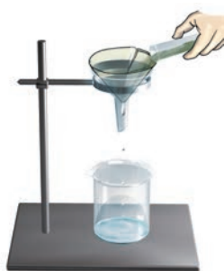
Fig. 5.10 Filtration using a filter paper
