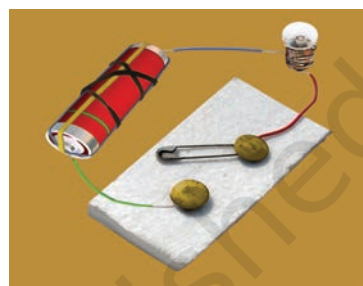
Fig 12.9 An electric circuit with a switch
