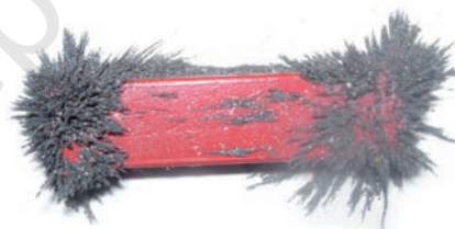
Fig. 13.7 Iron filings sticking to a bar magnet
