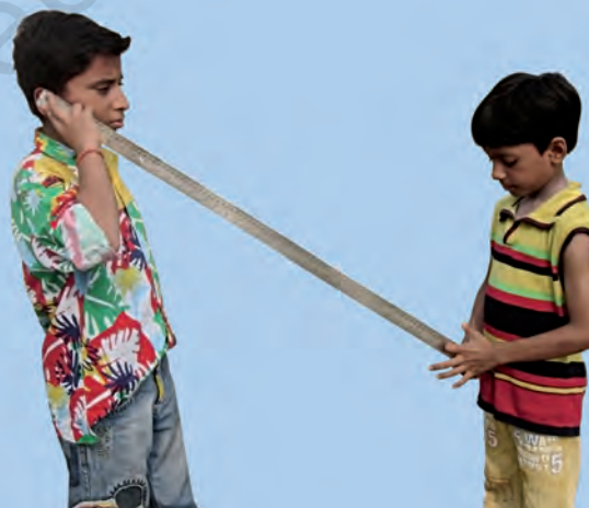
Fig. 13.12 : Sound travelling through a metre scale
