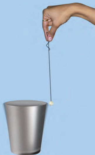
Fig. 13.17 : Thermocol ball touching the vibrating glass tumbler
