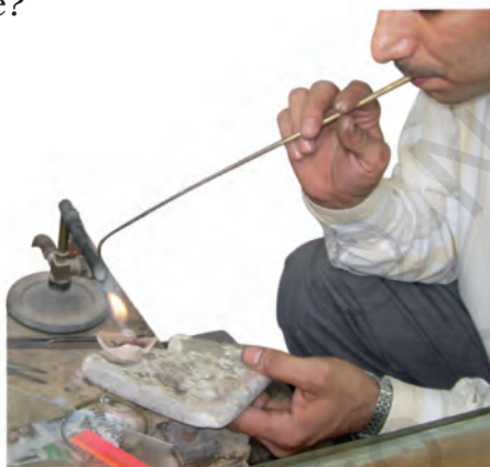
Fig. 6.14 : Goldsmith blowing through a metallic pipe
