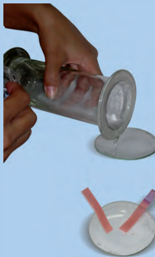
Fig. 4.4 (b) : Testing of solution with litmus papers
