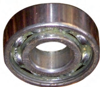
Fig. 12.16 : Ball bearings reduce friction
