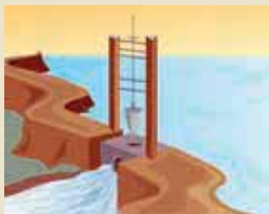
Sluice is a device to distribute the water from the water resources like river, tank and lakes. It is called Kumili, madai and Madagu in inscriptions.
