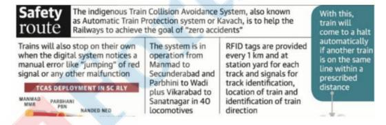
**Main Function of Kavach:** It is designed to bring a train to a halt automatically when it notices another train on the same line within a prescribed distance.
