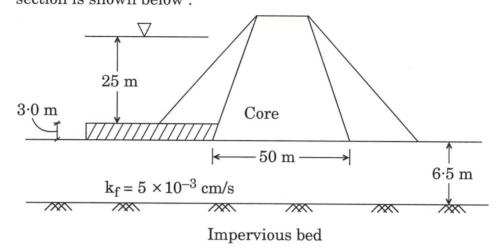
Also determine the seepage through the foundation after provision of Blanket. Also determine the head loss by the Blanket. Take permeability of Core/Blanket material as  $2\times 10^{-6}$  m/s. Permeability of foundation material is  $5\times 10^{-3}$  cm/s. Thickness of impervious blanket is  $3\cdot 0$  m.
